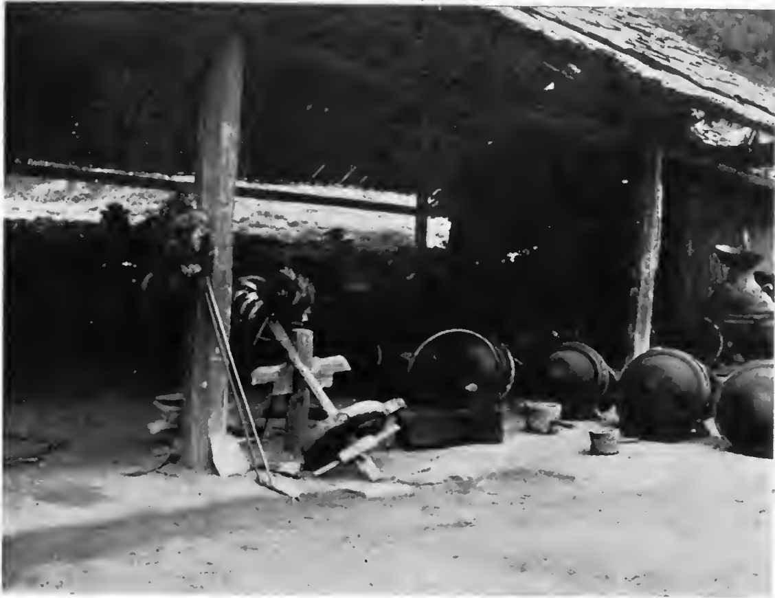
MOULD SHED OF AN IRON FOUNDRY (note piston of cylindrical blower).
